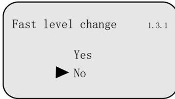
Move arrow with to Select Yes or No for Fast level change. Then confirm the selection with **OK**.
