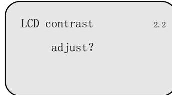
Adjust the B/W contrast by pressing **OK**, LCD Displays as below
