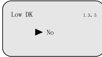
Push OK, enter the submenu of Low DK confirmation. LCD displayed below
