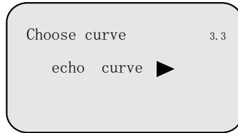
Pushing **OK** to select the curve. There are three curves: echo curve, False echo curve and Output trend curve .
