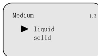
Move arrow with
