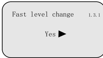
Push **OK** enter Fast level change confirmation. LCD displays as below
