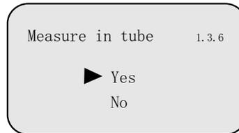
If the selection Yes is confirmed by OK, the diameter of the tube will be required. LCD displays as below
