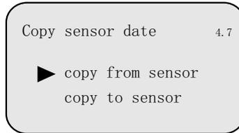
Copy from sensor means to save the sensor settings and copy to sensor means to restore the sensor settings.
