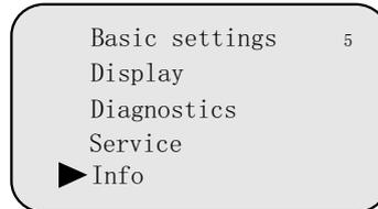
Then pushing **OK** enter the Info display menu. LCD displays as below
