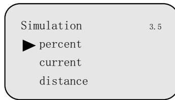
Pushing **↻** select the Simulation mode. Then confirm with **OK**. The corresponding value will be required and then simulation starts.
