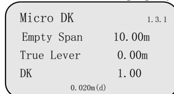
Normally when electronic constant is smaller than 1.4, the direct echo from the medium is low and hard to detect. However by measuring the echo reflected from the base of the vessel, the height of the medium can be measured. Two parameters are needed to be entered here.
